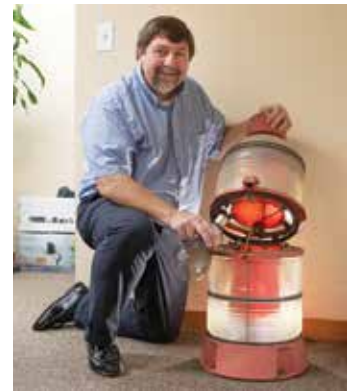
3ABN Radio engineer, Michael Babb, shows the old incandescent beacon recently replaced on WDQN’s tower.
